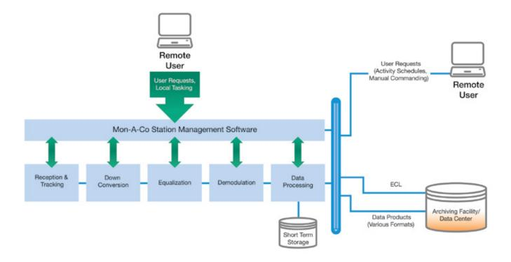
The ground station architecture makes it possible to operate the station locally via the user interface, or remotely via WAN. RF electronics are housed in the antenna structure to minimize losses.
