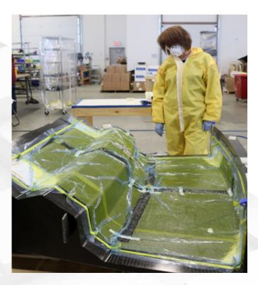
The vacuum infusion process is one of many closed-mold processes but is the only one that uses atmospheric pressure to push resin into the mold. This results in a controllable process because only three variables can affect the resin flow:
